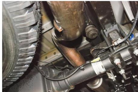
6. With proper clearance from spare tire install the exhaust tip onto the tailpipe. The system was designed to have the tip 1" below the quarter panel of the vehicle. With the tip in your desired position begin to tighten down all clamp connections from the
