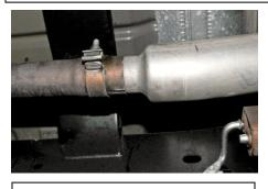
2. Install Headpipe #F onto the factory flange. You will re use the factory nuts at this connection. Loosely tighten down the flange.
