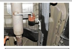
3. Install muffler assembly Item #A into the head pipe #F using clamp #E. Install hanger into rubber grommet and loosely tighten down the clamp. With the muffler assembly installed you may want to use a jack stand to support the muffler.
