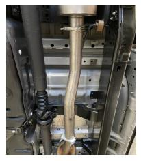
3. INSTALL HEADPIPE #A ONTO STOCK PIPE BEHIND RESONATOR. INSERT WELDED HANGER INTO RUBBER GROMMET. USE CLAMP #D PROVIDED TO SECURE. DO NOT TIGHTEN.
