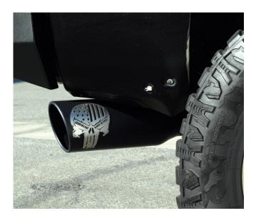
GIBSON EXHAUST systems are designed on a factory stock vehicle. Any aftermarket products installed could increase the sound levels of this Exhaust. Make sure there is a 1" clearance from ALL rubber brake lines, shock boots, fuel lines, tires, etc to prevent heat related damage or fire.
