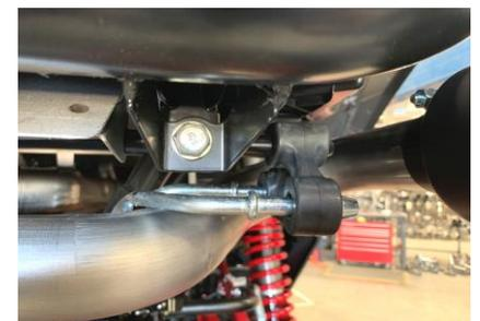
4. To install the Gibson muffler (Item A), re-install the factory rubber insulators on your new muffler assembly and install the muffler onto the factory hangers. Then install and tighten the flange bolts for the head pipe using Item G) included in the kit are shorter flange springs.
