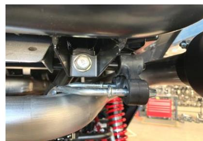
4. To install the Gibson muffler (Item A), re-install the factory rubber insulators on your new muffler assembly and install the muffler onto the factory hangers. Then install and tighten the head pipe using Item G) included in the kit are shorter flange springs.
