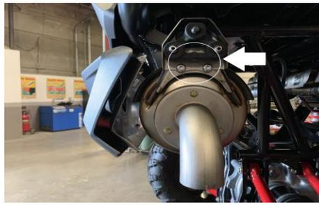
3. Remove the three bolts securing the hanger shield, then remove rubber insulator and then the shield. Next, remove the factory muffler by sliding it off the driver side hanger. Use WD-40 to lube the rubber insulators to aid removal.
