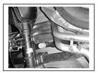
NEXT INSTALL DRIVERS OVER AXLE PIPE # D INTO MUFFLER 1<sup>1</sup>/<sub>2</sub> TO 2".USE CLAMP # F TO SECURE PIPE TO MUFFLER. DO NOT TIGHTEN. USE BOLT KIT # H TO SECURE PIPES TOGETHER. DRIVERSIDE TAB WILL BE ON THE BOTTOM.
