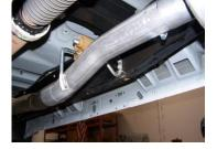
SECURE HEADPIPE TO FACTORY WELDED HANGER INTO RUBBER
