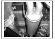
SLIP MUFFLER #B ONTO THE HEADPIPE 1 1/2" TO 2". THE OUTLETS WILL BE LEVEL. USE CLAMP #G TO SECURE MUFFLER TO HEADPIPE. DO NOT TIGHTEN.
