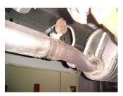
**1.** To remove the stock exhaust remove it from the second clamp located in front of the stock muffler. Disengage the welded hangers using WD-40 from the OEM rubber grommets. Do not damage or remove the rubber grommets as you will re-use them to mount your new system. Now, cut off tailpipe and remove
