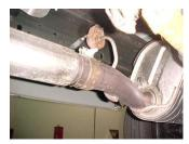
1. To remove the stock exhaust from the second clamp located in front of the stock muffler. Disengage the welded hangers using WD-40 from the OEM rubber grommets. Do not damage or remove the rubber grommets as you will re-use them to mount your new system. Now, cut off tailpipe and remove exhaust.
