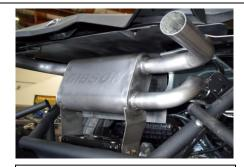
3. Install the Muffler Item A onto the factory muffler mount. Be sure the gasket has been reinstalled. RE install the factory hardware to support the muffler. Do not tighten.
