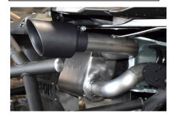
5. Install the Gibson exhaust tips to your desired look end length. You may need to loosen of the exhaust and re adjust to find the perfect position. Tighten down your Gibson exhaust tips securely.
