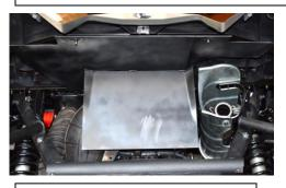
2. Install Item #B heat shield. Remove the 10mm bolts that attach the bed to the frame. You will use this hardware to mount the Gibson heat shield. Tighten and secure all hardware.
