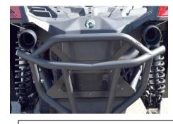
7. After your first couple runs double check clearance and re tighten all connections to prevent any movement caused by heat and usage of vehicle.
