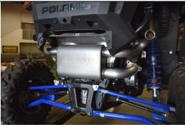
3. Next, install the Gibson Muffler assembly by removing the two bolts that secure the upper aluminum exhaust shield brackets to the frame. Slide the muffler hangers into the rubber isolators in the frame by tilting the top of the muffler forward to get it under the plastics then guiding the tailpipe brackets over the holes on the aluminum upper exhaust brackets. The brackets must remain in place before the installation of the muffler. Align exhaust studs into the 3-bolt flange while installing.
