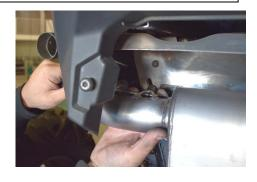
4. With the two bolts secure the tailpipe brackets to the aluminum upper exhaust shield brackets installed but loose, install the upper and lower factory springs back into their factory locations using a spring hook tool and or screwdriver.
