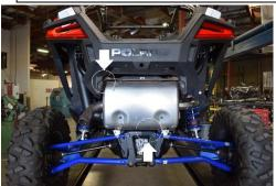
2. Remove the factory exhaust by un-bolting the factory rear shield that covers the muffler. You will re-use the hardware for the Gibson install. Disconnect the 2 factory springs and unbolt the
