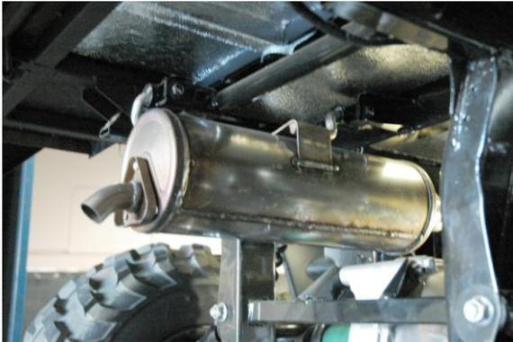
1. From underneath bed assembly, loosen both muffler clamps in front of the stock muffler assembly.
