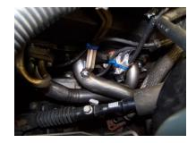
**6.** Using the supplied fasteners, bolt the Header to the bottom flange but do not tighten at this time. The nuts are jam nuts. Therefore they will not spin freely. This is normal. Torque headers to 30-35 ft/lbs after both headers are installed.
