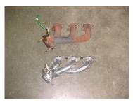
12.YOU CAN THEN INSTALL THE GIBSON HEADER USING SUPPLIED GASKETS AND HARDWARE. MAKE SURE TO USE ANTI-SIEZE ON HEADER BOLTS BEFORE INSTALLATION. TORQUE ALL HEADER BOLTS TO 30 FTS. THEN CONNECT EGR TUBE TO HEADER AND INSTALL SUPPLIED HEAT WRAP ON SPARK PLUG WIRES FOR BEST PROTECTION.
