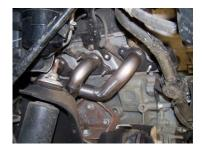
Now install Gibson Header and supplied gasket. Torgquing header to 30 to 35 fts torque.
