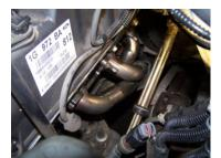
Now install driver side GIBSON header and gasket using stock hardware. (Make sure to remove stock EGR plug out of manifold and install it into Gibson header using some antiseizes!) Torque header to 30 to 35 fts. Now install, dipstick back on vehicle.
