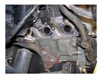
Remove manifold and stock gasket. Make sure to clean head surface of all debris before installation of header.
