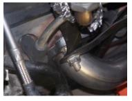
Now install driver side GIBSON header and gasket using supplied hardware. Also reuse stud and stock nut to remount dipstick tube and manifold bracket as shown in picture (Make sure to remove stock EGR tube out of manifold and install it onto Gibson header using some antiseizes!) Torque header to 30 to 35 fts. Now install, dipstick back on vehicle.
