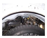
Start on passenger side its highly recommended to remove the inner-fender well to access the manifold. Loosen and set aside the transmission dipstick.
