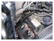
Now install Gibson Header and supplied gasket. Also re-use stock stud and nut of upper rear of cylinder head to mount manifold bracket as shown in picture Torque header to 30 to 35 fts torque.
