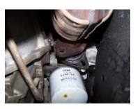
Re-Install Y-pipe assembly torque all fasteners to 30 to 35 fts torque. Then connect or sensor back in. Then start vehicle and check for leaks. Then after vehicle warms up let it cool down and re-torque all fasteners!
