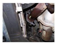
Re-install fender wall if removed. Use or Censored safe silicone on catalytic converter location if damaged in removal.
