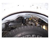
Start on passenger side its highly recommended to remove the inner-fender well to access the manifold. Loosen and set aside the transmission dipstick.
