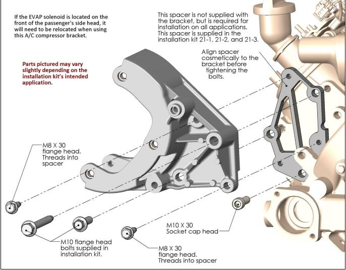
NOTE: Torque M8 bolts to 18 ft./lbs. and M10 bolts to 36 ft./lbs.
