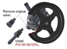
NOTE: If using AN fittings on the pressure line, Holley P/N 961961ERL AN extension/adapter is required.
