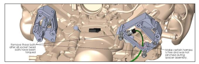
4. Install the accessory brackets per the instructions supplied with the brackets while substituting the below bolts supplied with the 21-5 installation kit. Sanden A/C compressor bracket shown.
