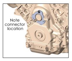
2. Install supplied harness assembly as shown. Make sure no wiring is pinched between engine and harness bracket. Reinstall the four harness bolts. Join the five connectors shown and engage red connector locks.
