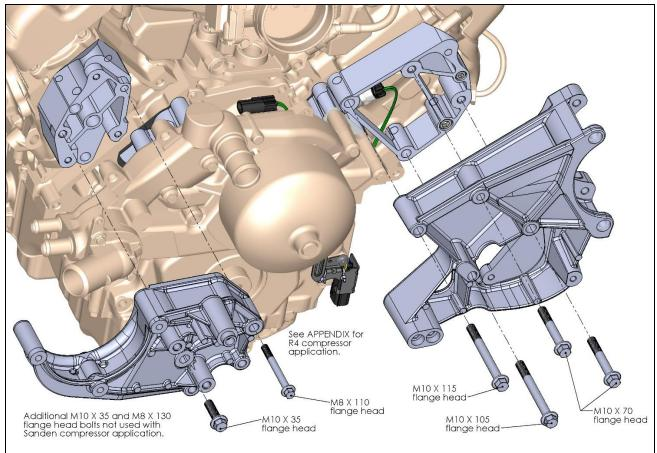
Torque M8 bolts to 18 ft./lbs. and M10 bolts to 36 ft./lbs.
