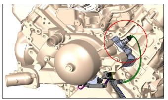
Torque temperature sensor to 15 ft/lb
