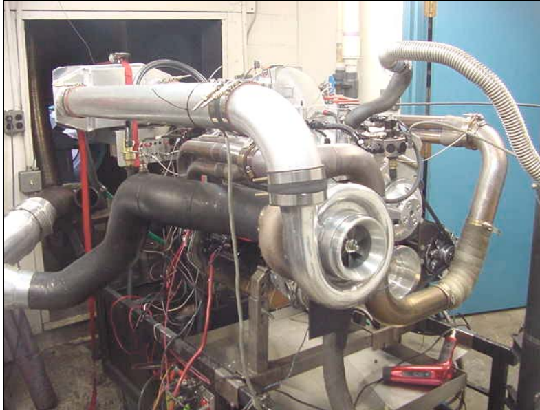
Figure 65 1500+ HP SBC Turbo Engine using Commander 950 PRO
