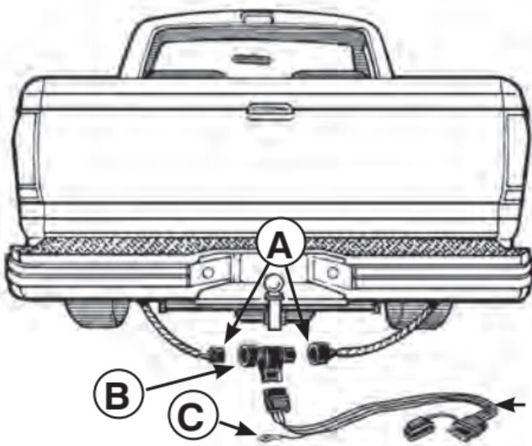
1. Locate vehicle taillight wiring harness (A). This harness will have the same connector end as the Wiring Kit. The most common location is 6" to 18" underneath vehicle behind the rear bumper near the driver's side frame rail.
