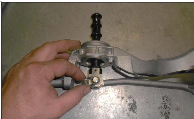
36. Apply a liberal amount of grease to the factory pins that connect the shifter housing and shift rod to the transmission.
