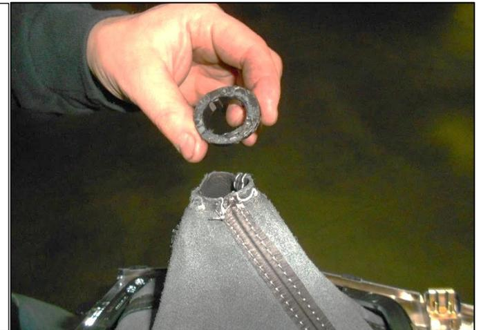
41. With the boot inverted, install the Hurst pistol grip shifter through the boot.
