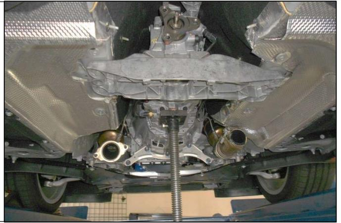
23. Remove the four 15mm bolts from the transmission cross member
