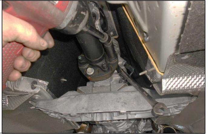
19. Remove the three 18mm bolts and nuts from the flex coupling and differential flange.
