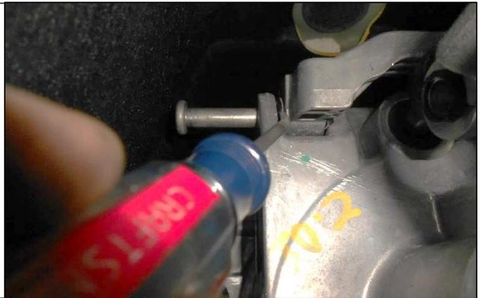
28. Remove the spring loaded clip from the cross pin that attaches the shift rod to the transmission and remove the pin.
