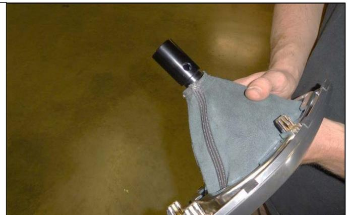
42. Ensure that boot is past the machined groove on the pistol grip and is orientated in the right direction. Secure the shift boot to the pistol grip using the supplied tie wrap.
