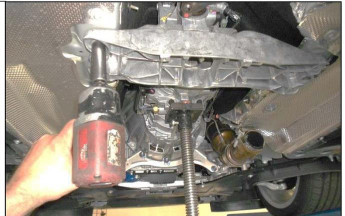
24. Lower the rear of the transmission enough to gain access to the front of the shifter housing.
