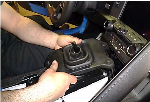
19. Remove the upper plate from the shifter.
