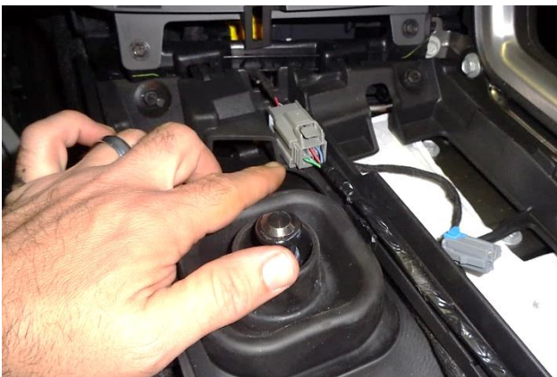
31. Reconnect the console harness plug at the front end of the center console, and check the security of the connection.
