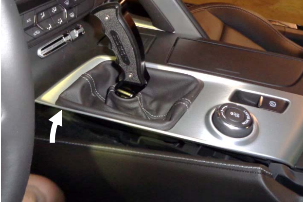
41. Reinstall the driver side trim panel.
