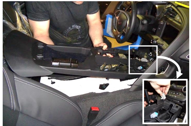
27. Carefully return the center console to the vehicle, situating the console harness plug in the notch at the front.
