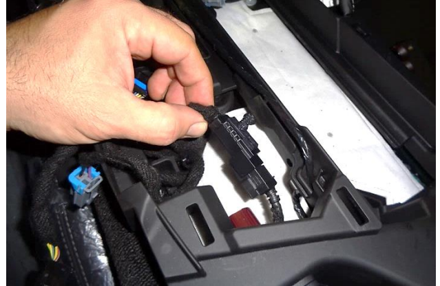
32. Reconnect the USB charger plug, and check the security of the connection.
