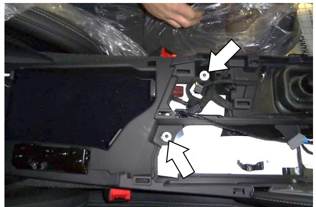
17. Remove the two nuts at the middle of the center console.
