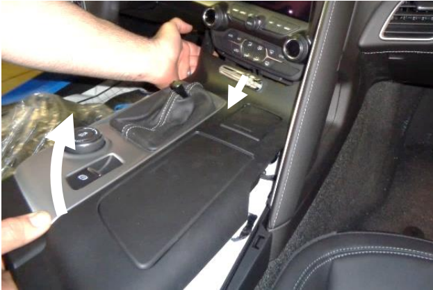
6. Carefully lift the back end of the panel while lowering the front end, to view the three electrical connectors underneath.
