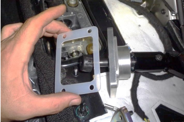
23. Install gasket (7) on the shifter pad.
