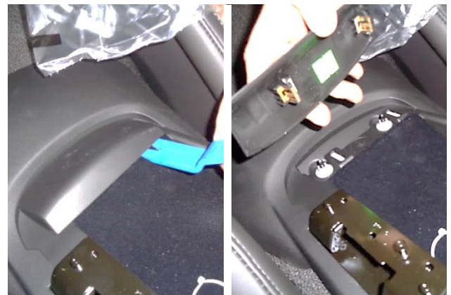
11. Use a plastic trim tool to remove the access cover at the rear of the center console.
