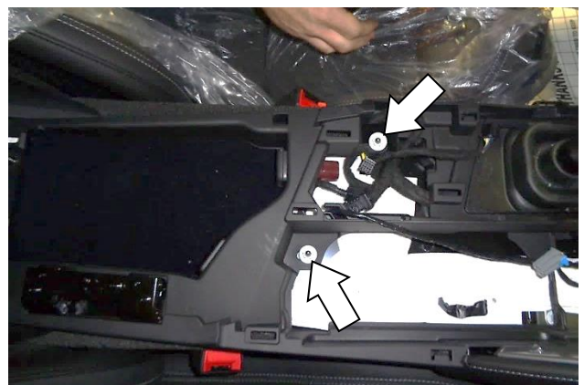
28. Reinstall the two nuts at the middle of the center console.
