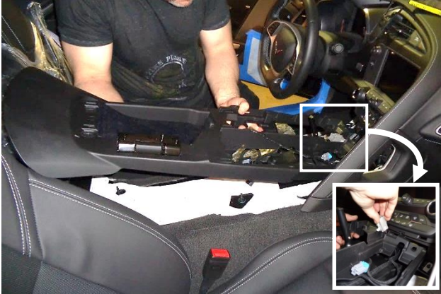
18. Release the console harness plug from the notch at the front of the center console, and carefully lift the console out of the vehicle.
