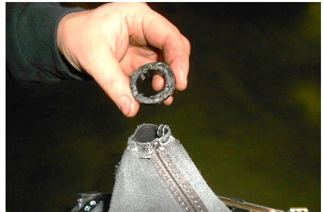
10. Remove the panel from the vehicle, then carefully pull the chrome collar off the inside of the shift boot. NOTE: The parts are glued together; use care not to tear the shift boot.
