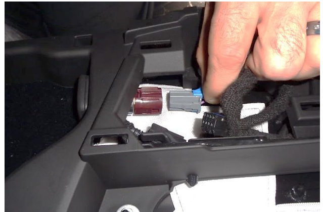
33. Reconnect the DC power connector, and check the security of the connection.
