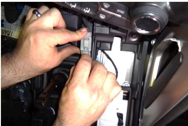
14. At the front end of the center console, disconnect the console harness plug.
