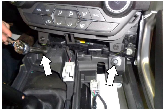
16. Remove the two bolts at the front of the center console.
