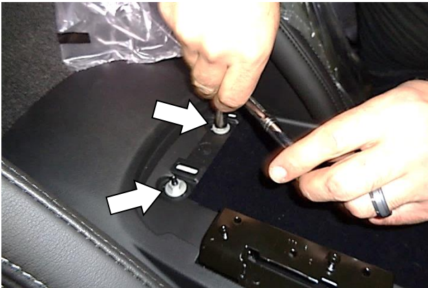
30. Reinstall the two nuts at the back of the center console.
