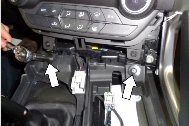
29. Reinstall the two bolts at the front of the center console.
