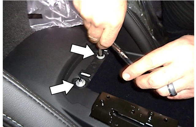
15. Remove the two nuts at the back of the center console.
