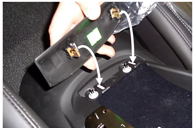
34. Snap the access cover back onto the rear of the center console.
