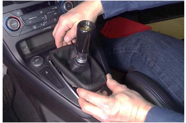
71. Snap the boot into the center console.
