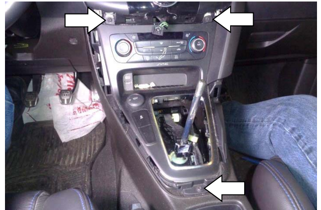
60. Install and tighten the 3 power panel screws.
