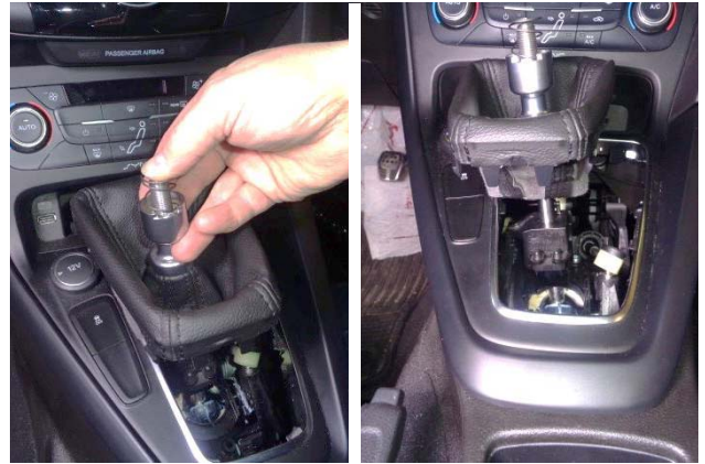
65. Move the shift lever into REVERSE gear.
