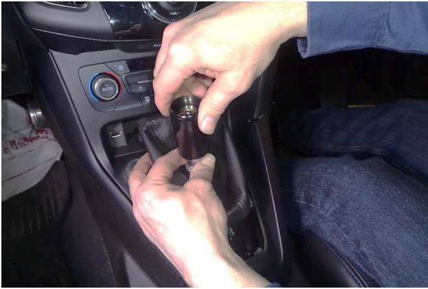
68. Thread the knob onto the lever. When it begins to drag against the reverse lockout collar, back it off approximately 1-1/2 turns.
