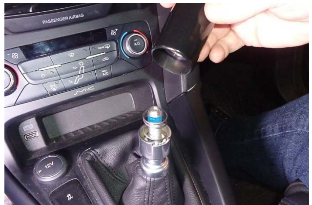
67. Apply medium strength thread-locking fluid to the first 4 or 5 threads on the shifter lever. CAUTION: Do not get thread-locking fluid on the reverse lockout return spring.
