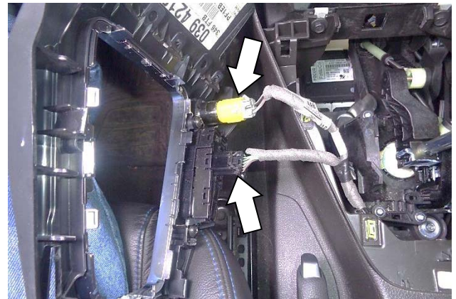
22. Disconnect the yellow (12V) and black (traction control) connectors.
