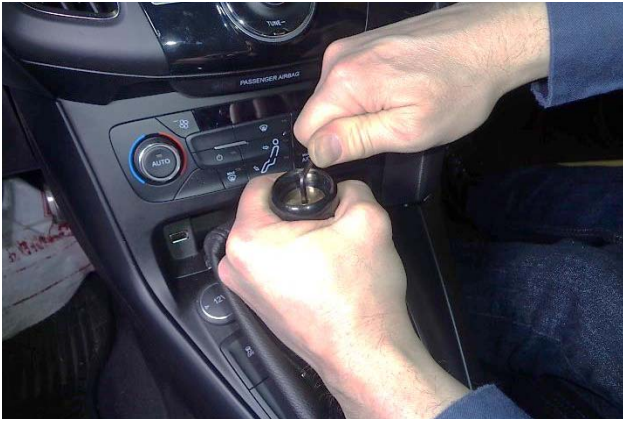
69. Firmly grasp the knob and tighten the set screw.
