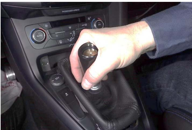
70. Move the shift lever into and out of REVERSE to verify correct operation of the reverse lockout. The reverse lockout lever should lift just high enough to clear the lockout notch on the shifter housing without touching. Adjust the height of the shift knob if required.
