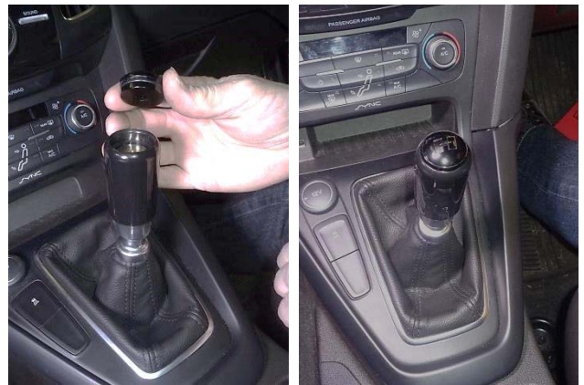
72. Lightly grease the O-ring (2) and install it on the cap (1). Then align the logo as desired and press the cap into the knob. Go to Step 76.
