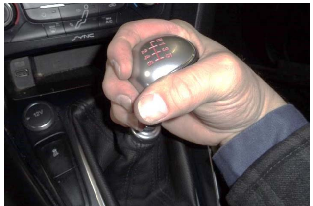
73. TO USE STOCK SHIFT KNOB: Thread the knob onto the lever. NOTE: The knob's threads are tapered, so more turning force is required the further it is installed.
