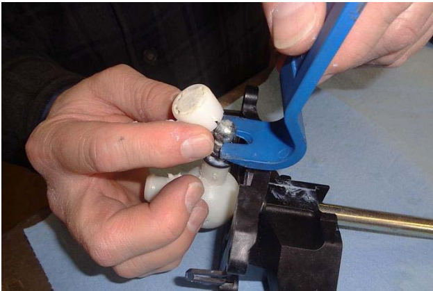
32. Pull the side pivot cup off of the side pivot ball.
