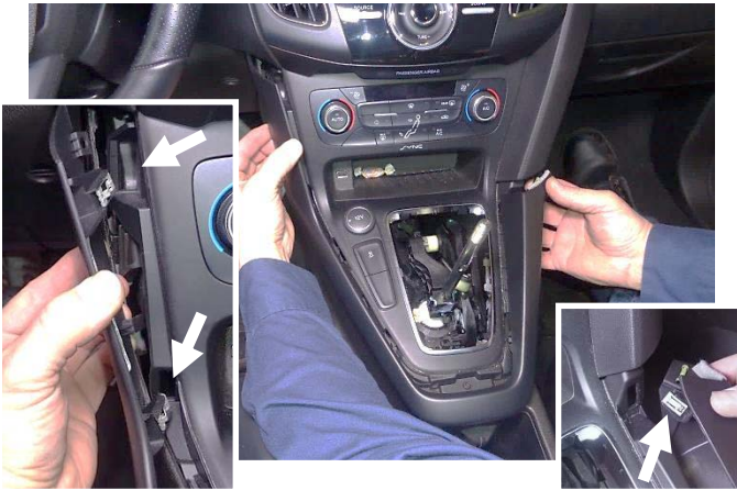
14. Use a trim tool to remove the trim that wraps around 3/4 of the shift console. Note that there are 2 spring clips on the left, and 1 spring clip on the right.
