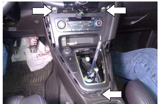
18. Remove the 3 power panel screws.
