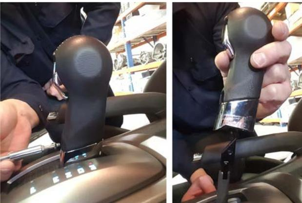
3. Remove screw from front of shifter handle then remove handle.
