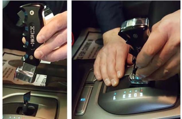
4. Install assembled shifter handle (1).
