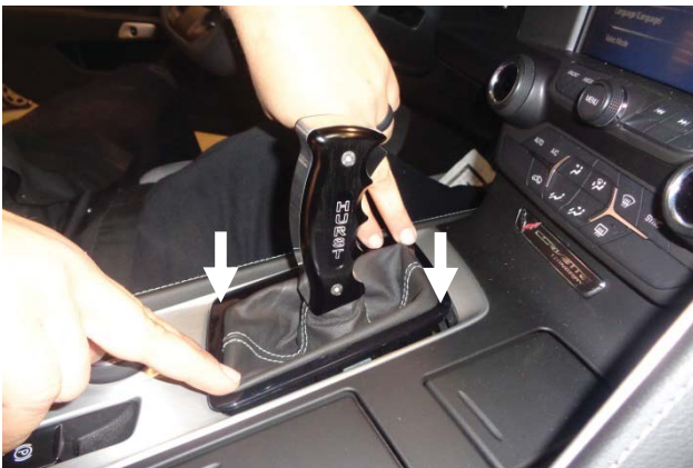
15. Snap the bezel back into the center console.
