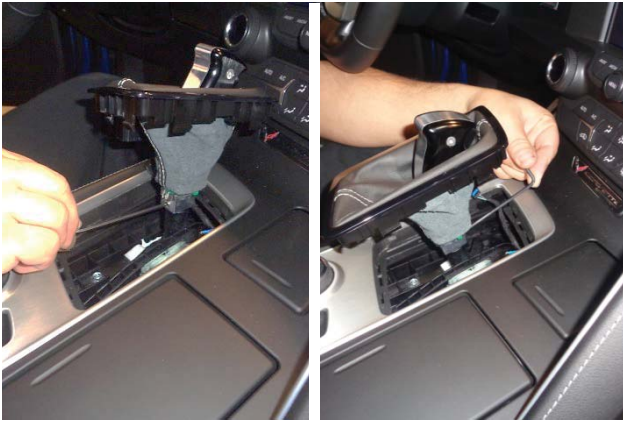
13. Tighten the set screws. (Pull the shifter back to reach the front screw, if required.)
