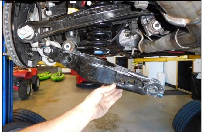
9. Once the spring moves freely, remove the jack and let the rear control arm swing out of the way, while holding onto the spring.
