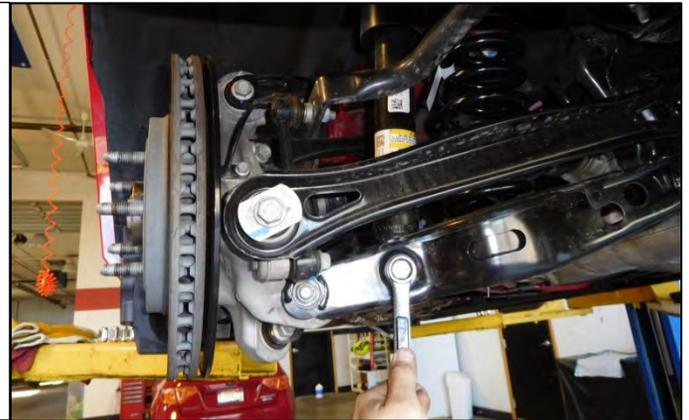
5. Loosen the bolt that connects the hub assembly to the rear lower control arm.
