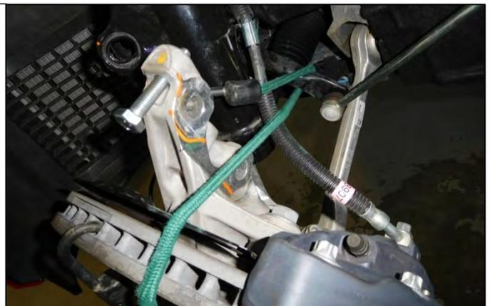
22. Support the strut assembly and remove the three strut tower bolts loosened in the previous step, then remove the strut assembly. Pay close attention to brake and ABS lines when removing the strut assembly, making sure not to snag them.
