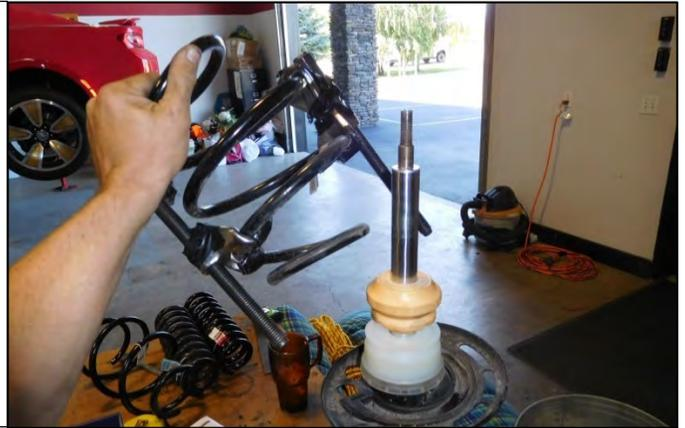
28. Install your new Hurst spring in the reverse order of removal. Take note of the rubber isolator on the strut assy. Align the new spring making sure it seats properly.
