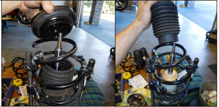
27. Remove the spring. Carefully loosen the spring compressors until they can be removed from the spring.
