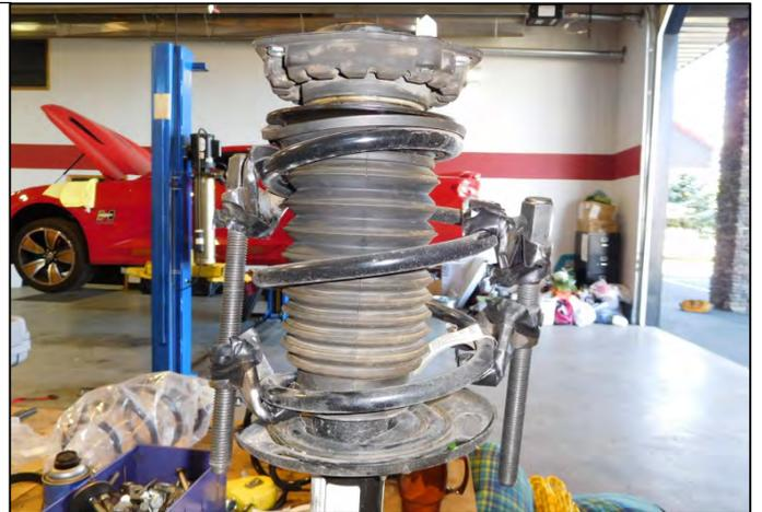
25. Once the upper cup no longer has tension from the spring, remove the nut holding the upper cup in position. A strap wrench may be needed to hold the shaft of the shock to allow the locking nut to be removed.
