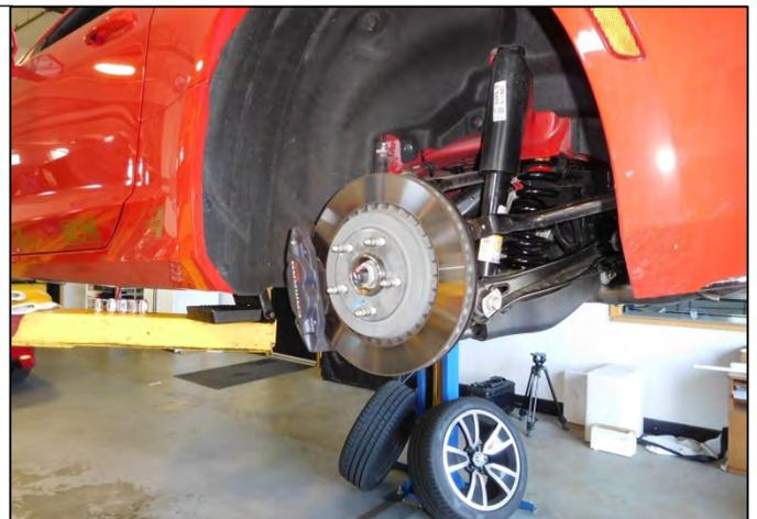
2. Remove the four plastic rear clips that mount the plastic control arm covers by pushing down on the center pin, then remove the covers.
