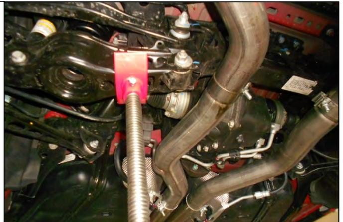
4. Remove the lower bolt from the rear shock.
