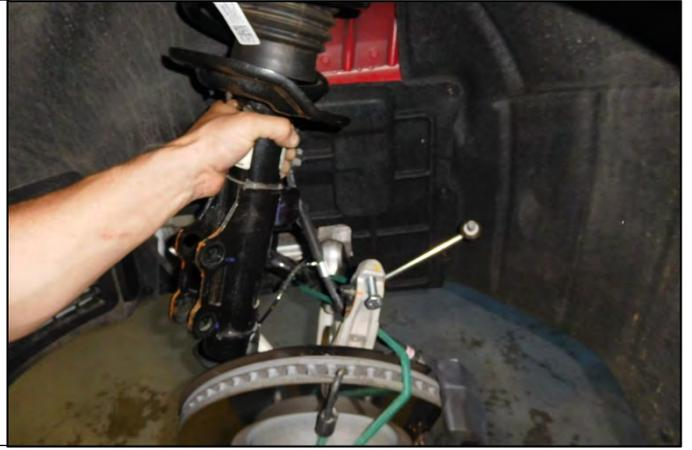
23. Remove the rubber cap from the top of the strut, exposing the nut. The nut will be removed in a later step.
