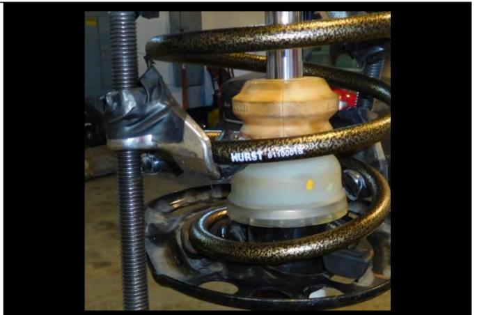
30. Also note that the upper cup assembly has no special alignment for the top of the spring. The upper cup assembly can be installed without any alignment marks.
