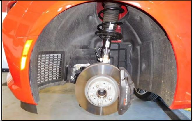
15. Install a M10/1.50 bolt into the upper portion of the spindle assembly until it makes contact with the strut. Use a nut to lock the bolt into position. This sets the alignment angles for re-assembly. Vehicle alignment is still needed.
