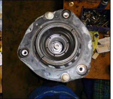
24. With the strut assembly supported, use spring compressors to remove tension from the upper cup of the strut. Springs are under extreme tension. Great care should be taken to ensure safety. If using compressors like the ones shown in the image, tighten them evenly from side to side.
