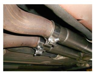
5) Begin the installation by placing a supplied 2-3/4" clamp onto each of the inlets of the X-pipe assembly **#26578M.** Then, place the X-pipe onto the back of the stock head pipes (the embossed Hurst H will be facing the ground). Level and center the assembly in the drive line tunnel and support with a stand. Tighten the two clamps enough to hold, but still allow for adjustment.
