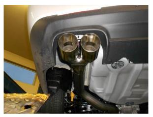
7) Place a supplied clamp onto the left muffler outlet. Place the left tailpipe #26637M into position and starting from the rear, connect the hangers on the tailpipe to the rubber mounts on the vehicle. Slide the tailpipe fully into the muffler outlet. Adjust the tailpipe so that the stainless tip is level and centered in the bumper cut-out. Tighten clamp enough to hold, but still allow for adjustment. Repeat this step for right tailpipe #26635M.
