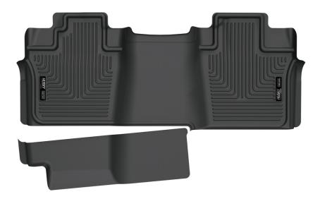
IF YOUR VEHICLE IS EQUIPPED WITH A FACTORY SUBWOOFER LOCATED UNDER THE DRIVER'S SIDE REAR SEAT, YOU WILL NEED TO TRIM YOUR LINER TO ACCOMMODATE THIS OPTIONAL FEATURE. TO TRIM THE LINER, USE THE LOWERED STEP IN THE PART LOCATED BEHIND THE RAISED RIB-WALL AS YOUR TRIMMING GUIDE. CONTINUE TRIMMING OVER THE HUMP USING THE STEP IN THE PART AS YOUR GUIDE.
