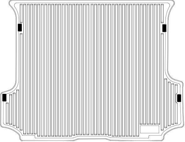
TO ACCESS THE FACTORY CARGO TIE DOWN HOOKS WITH YOUR LINER IN PLACE, TRIM AWAY THE MATERIAL FROM THE FOUR RAISED AREAS ON YOUR LINER (SHOWN ABOVE DARKENED) LEAVING THE RAISED EDGE. A UTILITY KNIFE WORKS WELL FOR TRIMMING.
