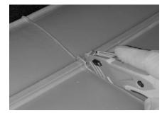
Where applicable, feed the strap through the liner that used to lower your third row seats. Vehicles with power folding rear seats will not have the straps.
