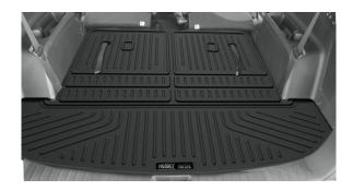
5. The first time the rear seat backs are moved to the upright position, move the seats slowly taking care to ensure the accordion section of the liner folds outward as shown. This may need to be assisted from the backside.
