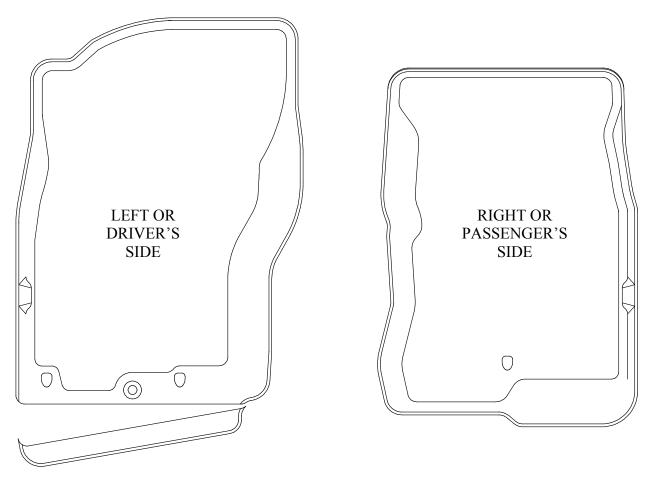
IF YOUR VEHICLE HAS THE OPTIONAL FACTORY SUBWOOFER MOUNTED UNDER THE FRONT DRIVER'S SIDE SEAT, YOUR LINER WILL NEED TO BE TRIMMED TO ACCOMMODATE THIS OPTION. TO TRIM, USE A UTILITY KNIFE OR HEAVY SHEARS REMOVE THE REAR PORTION OF THE DRIVER'S SIDE LINER AS SHOWN IN THE DIAGRAM. THERE IS A MOLDED IN TRIM STEP IN THE PART TO AID IN TRIMMING.
