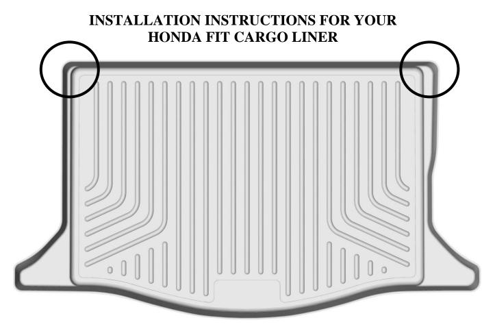
TO MORE EASILY ACCESS THE FACTORY CARGO TIE-DOWN HOOK LOCATIONS WITH YOUR LINER IN PLACE, YOUR LINER HAS TWO TRIM AREAS LOCATED ON THE BACK WALL (SEE CIRCLED AREAS ON DRAWING ABOVE). THE AREAS THAT CAN BE TRIMMED ARE LOWERED IN THE PART AND CAN EASILY BE TRIMMED WITH A UTILITY KNIFE OR HEAVY SHEARS.
