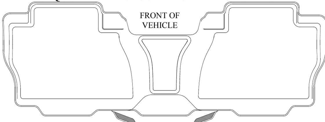
Trimming is needed to allow the correct fit for vehicles **with** 2<sup>nd</sup> Row Bench seats. To trim, remove the two areas along the back wall of the liner shown above darkened. Use the molded in step and groove in the part as your trimming guide. A utility knife or heavy shears work well for trimming. You will find photos the trimmed part on the back of this page.
