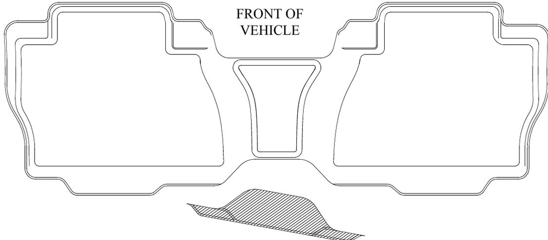
Trimming is needed to allow the correct fit for vehicles **with** 2<sup>nd</sup> Row Bucket seats with a 2<sup>nd</sup> Row Console. To trim, remove the area along the back wall of the liner shown above darkened. Use the molded in groove in the part as your trimming guide. A utility knife or heavy shears work well for trimming. You will find photos the trimmed part below.
