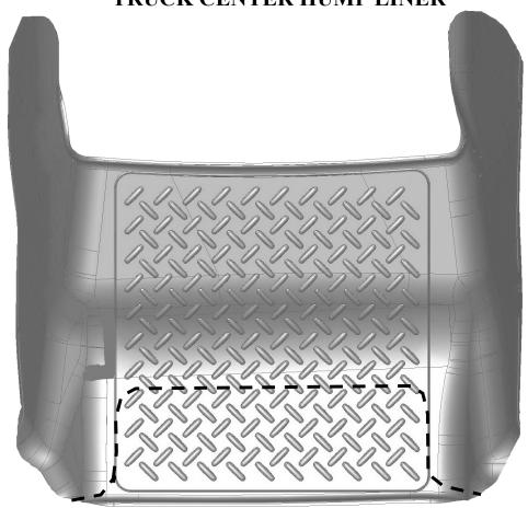
IF YOUR TRUCK HAS FRONT ROW BUCKET SEATS WITH A FACTORY CONSOLE BETWEEN THEM, YOU WILL NEED TO TRIM YOUR LINER TO ACCOMMODATE THE CONSOLE. TO TRIM, SIMPLY USE THE RECESSED STEP IN THE PART AS YOUR TRIM GUIDE AND REMOVE THE LOWER PORTION OF THE LINER. THE DOTTED LINE ABOVE APPROXIMATES THE STEP MOLDED INTO THE PART.
