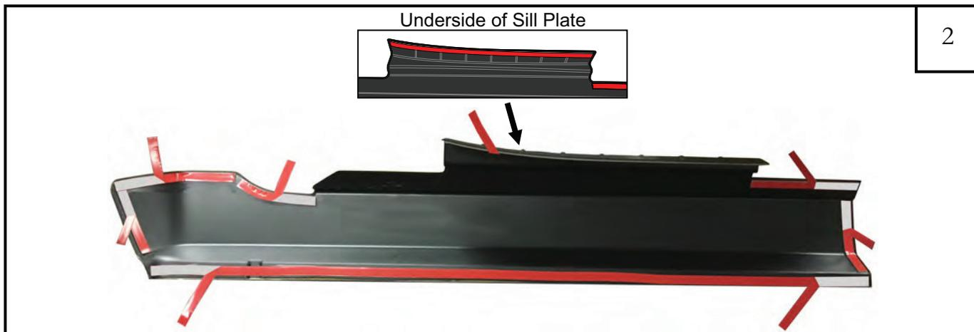
Open vehicle doors. Clean all dirt and debris from vehicle door sills and rocker panel. Use supplied alcohol wipes where part will attach.
