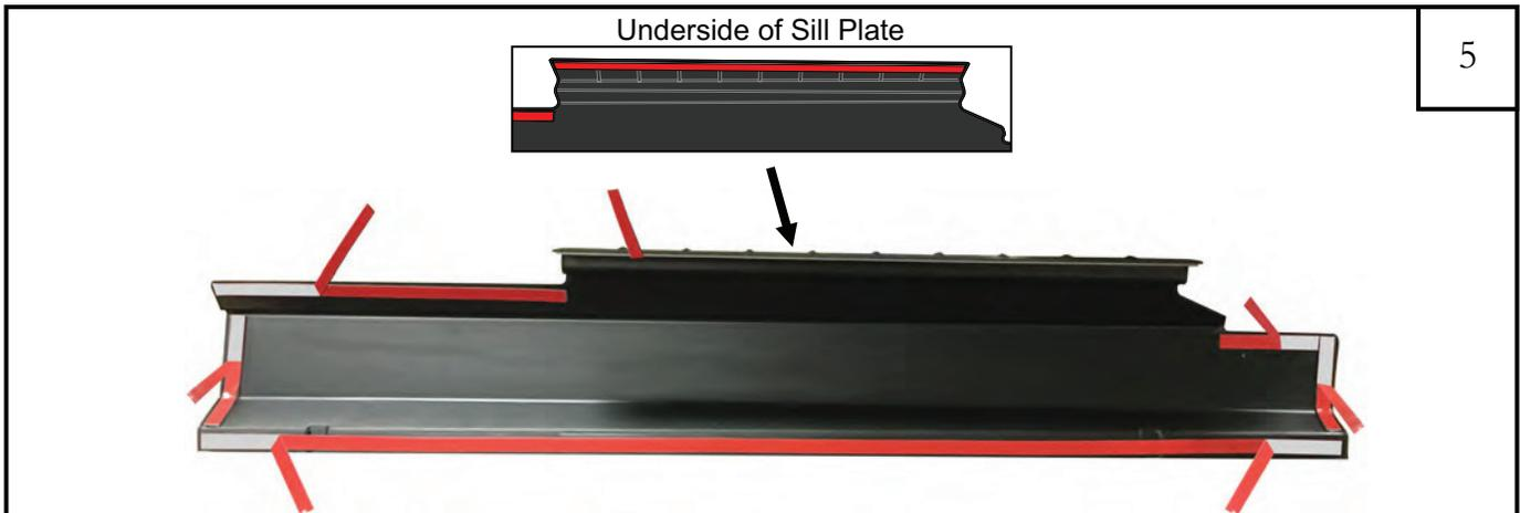
Peel back roughly 3" of red tape liner from the pieces of tape on the back side of the front part. Make sure red tape liner will be accessible when part is attached to truck.
