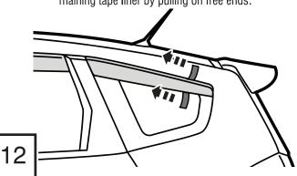
Apply pressure along all flanges to ensure proper adhesion of tape.
