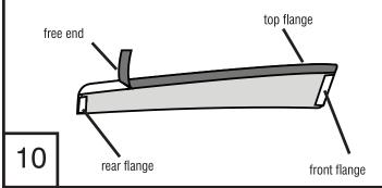
Align the deflector on the outside of the door frame. Align the front of the Extended rear Visor parallel to the previously installed Rear Visor.
