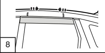
Apply ressure along all flanges to ensure proper adhesion of tape.
