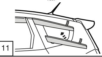
Gently press the exposed areas of tape against the surface and verify position. With the visor in its final position, remove the remaining tape liner by pulling on free ends.
