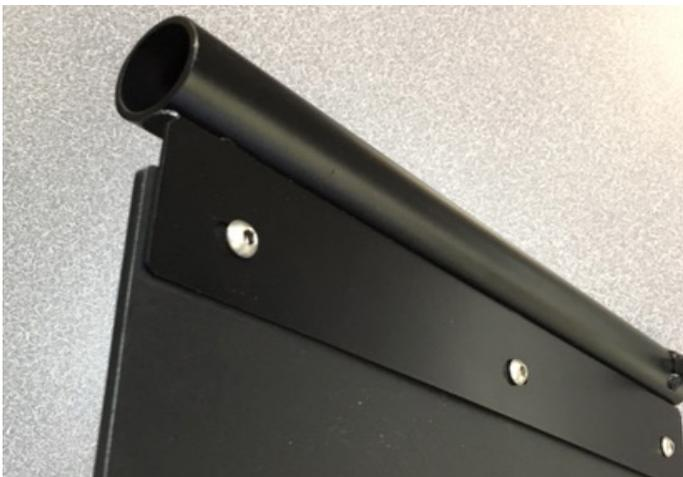
2. Assemble the upper flange bracket with the SS button head cap screws through the flange, mudflap, washer and into the nyloc hex nut.
