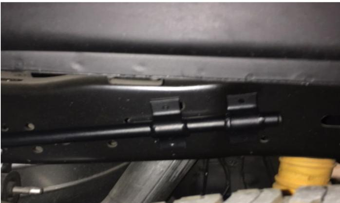
3. Find the proper mounting location for the mounting bar by holding the bar and mud flap in the wheel well opening.
