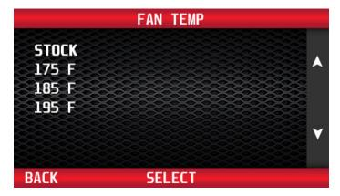
Use the buttons to the right of the screen to select the desired temp thermostat. Press 'Select' to save the chosen themostat temp.
