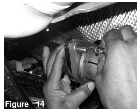
Figure 14 Use two m10 bolts and flange nuts to connect the test pipe and the primary section together.
