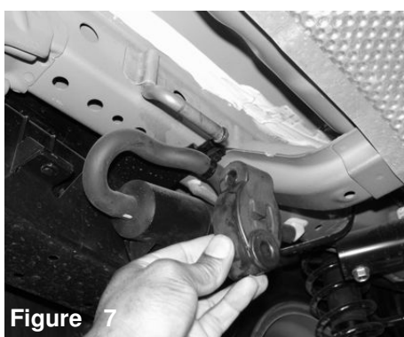
Figure 7 Driver side rear hanger: Once you have removed lower pin from the grommet, continue to remove the grommet.
