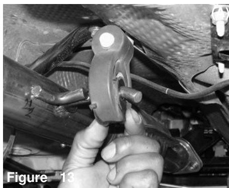
Figure 13 The primary section hanger is inserted into the stock grommet.
