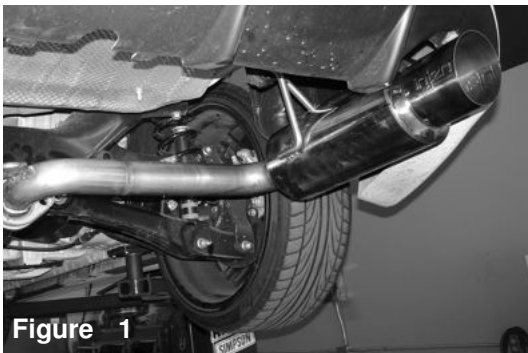
Figure 1 60mm high flowing exhaust system with catalytic converter, titanium tip and test pipe.
