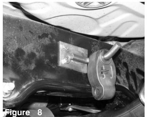
Figure 8 The grommet is placed over the new bracket as shown above.
