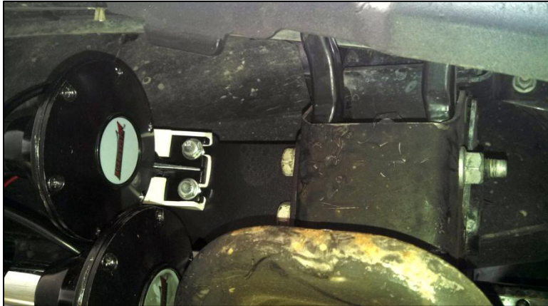
Figure 5: Horn Mount Installed with Tow Hook:
