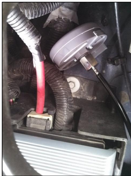
Figure 3: Remote Filter Mount Behind Fusebox:
