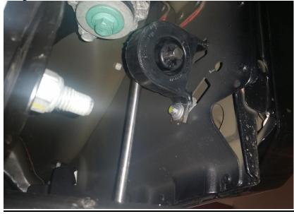
**STEP 4.** Slip side exit exhaust pipe onto extension (or muffler if Super Cab) using 3" band clamps and slide into both hangers.
