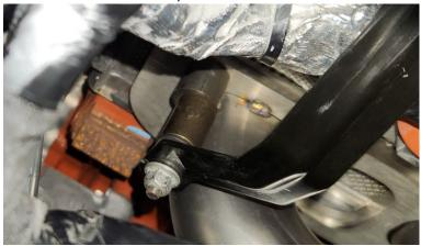
Move to top driver side of engine. Install supplied dip stick spacer brackets (K60901 and K60902) and supplied hardware onto top of valve cover, oil fill tube, and dip stick. K60901 bolts to valve cover using OEM bolt and to dip stick using M6x1 – 15mm bolt and M6 Nylon nut. K60902 bolts to oil fill tube using M8x1.25 – 20mm bolt and to dip stick using M8x1.25 – 20mm bolt and M8 Nylon Lock Nut. Should look like image below-
