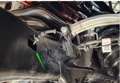
Using bracket (K60903) and supplied hardware (M8x1.25-20mm Bolt and M8 Nylon Lock Nut), bolt bracket into hole located above sway bar mount on frame. Route wiring under bracket. This will keep wires away from primaries. Should look like image below-
