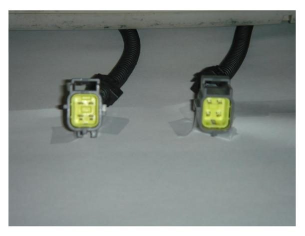
Daimler Chrysler SRT-8 O2 Extensions, the black front O2 extension may need to have the top tab ground off and on the rear gray O2 extension the offset tab may have to be ground off also\*
