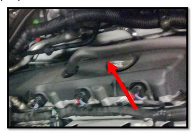
• Using a small flathead screwdriver, pop out the retaining clip located on the valve cover vent port. The other end of the hose can be removed by squeezing the connector lock and pulling out the PCV valve.
