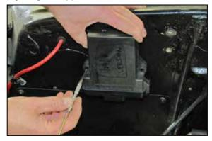
2. Find a suitable location to mount the ECI control unit that is away from direct heat, wet conditions and any mechanical interference. Place the control unit in position and mark the location for holes to be drilled.
