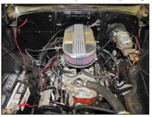
9. Reinstall the air filter assembly.
