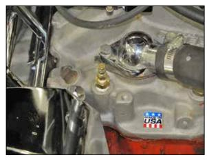
8. If you desire to connect a coolant temperature sensor to the system, find a suitable location in the cooling system to install the coolant temperature sensor. Usually this will be in the intake manifold near the thermostat housing.
