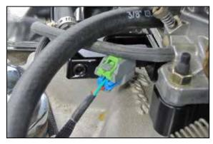
5. Route the wiring pigtails for the injector(s) and other optional connections so they will not interfere with mechanical assembly or exhaust and then connect them to the injector(s) and optional locations.
