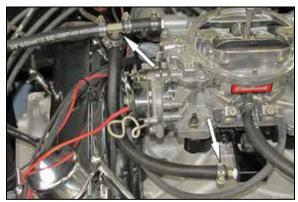
7. Install a TEE into the fuel line. Using a suitable fuel hose, connect the TEE to the injector supply.
