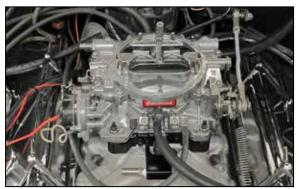
6. Install the carburetor and reconnect the throttle linkage, vacuum lines and electrical connections.
