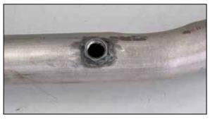
4. Weld the provided O2 sensor fitting into the exhaust pipe.
