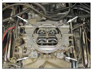
2. Remove the bolts that secure the carburetor to the intake manifold. Remove the carburetor and gasket from the manifold.
