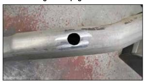
3. Drill a  $\frac{3}{4}$ "id hole in the marked location. Deburr the hole after drilling.
