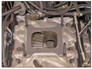
3. Be sure that the mounting flange on top of the manifold is clean and dry. Install the provided extended carburetor studs and new base gasket onto the manifold. Be careful that no debris falls into the manifold as SEVERE engine damage may result.
