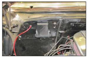
3. Drill the holes and mount the control unit in the desired location.
