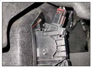
2. Locate the pedal wiring harness connection on top of the throttle pedal assembly and release the locking tab and disconnect the electrical connection. Disconnect the Throttle pedal electrical connection.
