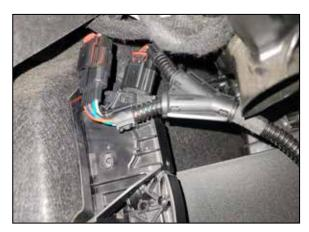
3. Connect the K&N throttle harness to the throttle pedal and connect the factory harness to the K&N harness. Note: There are 2 harnesses included with this kit, use connector that matches your vehicle's connector.
