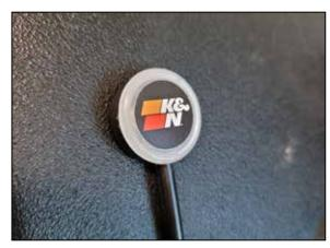
5. Route the illuminated button to desired locaation where it can be easily pressed without obstruction. Wipe surface clean for button to be mounted with alcohol/glass cleaner to ensure proper adhension. Pull ogg adhensive backing and firmly press button onto surface.
