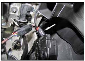
3. Connect the pedal module wiring harness into the pedal assembly and then connect the factory wiring harness into the pedal module wiring harness.
