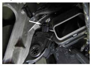
2. Locate the pedal wiring harness connection on top of the throttle pedal assembly and release the locking tab and disconnect the electrical connection.
