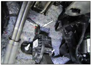
2. Locate the pedal wiring harness connection on top of the throttle pedal assembly and release the locking tab and disconnect the electrical connection.
