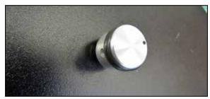
4. Find a suitable location to mount the sensitivity knob, drill a  $\frac{1}{4}$ "id hole, remove the knob and install the rheostat then reinstall the knob.
