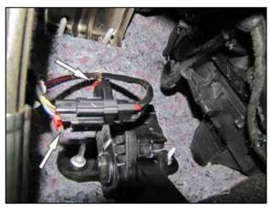
3. Connect the pedal module wiring harness into the pedal assembly and then connect the factory wiring harness into the pedal module wiring harness.
